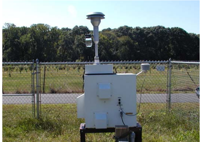
Figure 1: Ambient air monitoring fine particle sampler located at the New Brunswick Site in Middlesex County.
